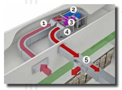
• The DryComfort unit draws warm, humid room air into the heat exchanger, transferring sensible heat to the heat exchanger. Cooled, moist air moves to the dehumidification coil.
