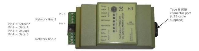
The Modbus adaptor is also available in a DIN rail mounted enclosure, connections are the same as the PR0623 adapter shown above.
