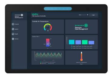
The TouchXL, when connected to the Intuitive, is used as a display, mimicking the view of the standard web interface to the controller. It is used to interact with the application software and alarm indication (if programmed into the TDB).
