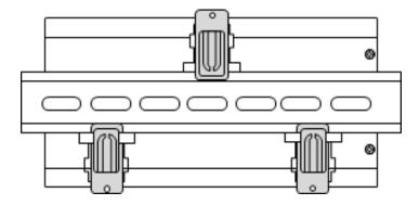
The controller can now be pushed flat onto the DIN rail and the top foot pushed in 2 clicks to hold the controller in place. Finally, push the bottom two feet in by one click to secure the controller.
