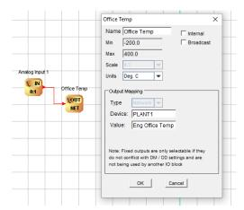
A simple Data Builder PLC program, running on a Data Manager, is shown on the left. The temperature of a room is being measured from probe 1 on the Data Manager's analogue input board and is being mapped to an analogue output. By right-clicking on the 'Analogue Output' block, in the Data Manager TDB program, the properties window on the left is shown. This block has to be configured so that values can be sent to a TDB controller.
