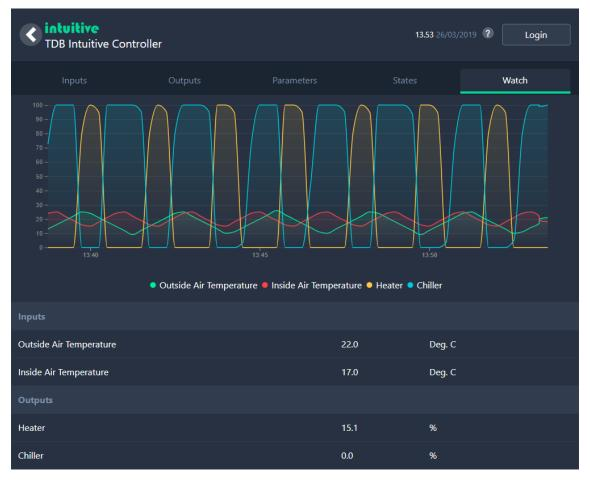
The graph will automatically scroll, refreshing the data every 15 seconds and will show traces over a 15 minute window. The graph is time stamped and the user can also temporarily hide certain traces by clicking on the name of the control value beneath the graph.
