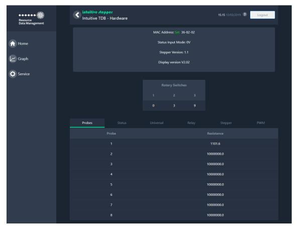
As shown in the above screen shot viewing Hardware allows the user to check IO values for test purposes. It also provides a general overview of any other hardware setup, for example if the unit is logging to a memory stick or if there is a plant USB Touch screen attached.
