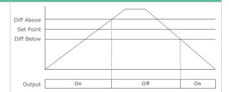
Reverse On/Off blocks are typically used to control a heating function.
