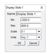
The Display Slide Block can be used in conjunction with either the Plant Touch Screen Display or the layout option within the web/ TouchXL interface.
