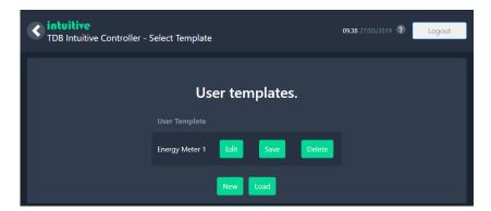
Following the creation, the template can be saved to a local PC, using the 'Save' button. The format will be saved as an xxxx.typ. When saved, the template can be re-used on other devices as long as the User Template feature is activated.
