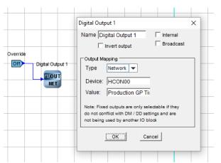
Shown on the left is a simple software manual override. This has been generated in a Data Builder program running on a Data Manager. By right-clicking on the 'Digital Output' block the properties window on the left is shown.
