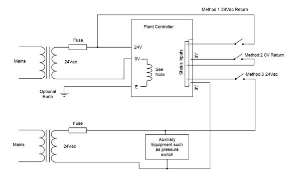
**Note:** Current versions of Plant hardware have 0V and Earth linked internally via an inductor, this is recognisable by Status LED. See diagram on page 9 for location of status LED
