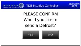
If the left hand response button ('YES') is pressed then the 'Yes Button' output is momentarily activated. If the right hand response button ('NO') is pressed then the 'No Button' output is momentarily activated.
