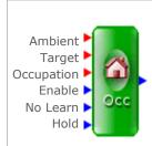
The Occupancy Optimisation block is used as an energy saving tool. The block calculates when to enable the output, connected to the heating/cooling strategy, to achieve the desired room temperature for when the room is first occupied.
