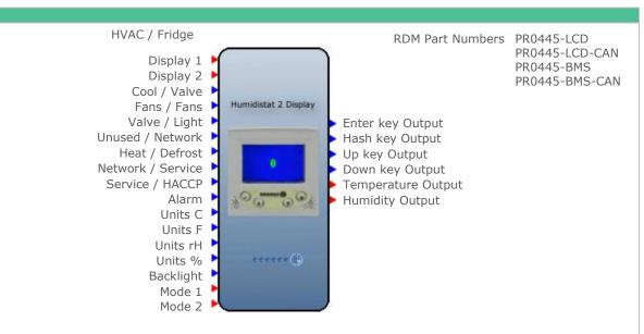
The Humidistat 2 display comes in two different hardware variants; **Fridge (PR0445-LCD)** or **HVAC (PR0445-BMS)**. Therefore within the display block properties (below), the user must define which 'Type' is being used. If the hardware and the selected type is mismatched, the functions will not work. **Note**: changing the type will dictate the input aliases as listed above.
