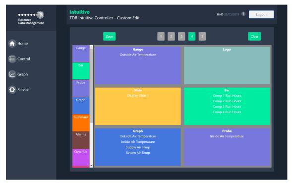
The icons listed on the left of the viewing pane can be dragged and dropped to the desired location. Once placed, the individual sections can be edited by double clicking on them. Depending on the selected widget the options to configure it will differ. Details are below.
