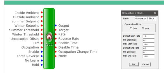
The Occupancy Optimisation block 2 is used as an energy saving tool. The block calculates when to enable the output, connected to the heating/cooling strategy, to achieve the desired room temperature for when the room is first occupied.
