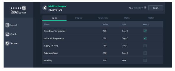
The Control Summary will list all Inputs, Outputs, Parameters and States which have been configured within the TDB program. It will also feature a Watch tab.
