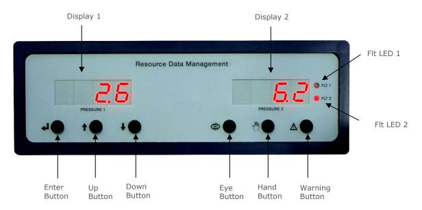
When using the remote plant display, if the number sent to the display is greater than 999.9 then the decimal part of the value is dropped and replaced with a thousand digit e.g. 999.8, 999.9, 1000, 1001, 1002 and so forth. When the display is connected to the controller but not utilised in the TDB program it will show 'b 28' when the controller is powered on.
