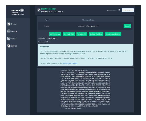
The lines of text generated is what's required to be sent to the Certificate Authority (CA), therefore copy and paste the code into a text file and send it direct to them.
