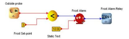
The above diagram shows a simple Data Builder application for a frost alarm. An outside temperature probe is connected to an analogue input and this is compared to a frost set-point. If the temperature goes below this set point (using a less than block) the output of the less than block goes on. This goes to the alarm block that has a delay of 10 minutes. If the signal is still on after the 10 minutes, the relay will be energised.
