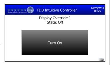
When the button is pressed, the description will change to 'State: On' changing the output of the block to 'On' and the text inside the button will be 'Turn Off'
