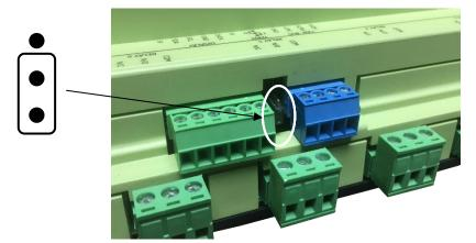
The end of line termination resistor link should be fitted to the middle and bottom pins on the Main control board and on the last expansion board on the CANbus network. All other expansion boards should have the link removed or fitted to the middle and top pins.
