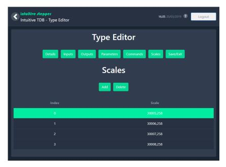
Once created, the scaling values taken can be applied to the values by using the method described in the variable scaling section. The scales, as mentioned can be referred to by using \$0, \$1, \$2, \$3.
