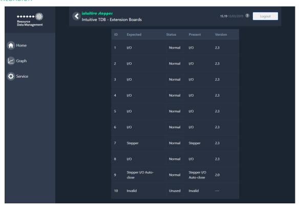
The Extension page will list the current expansion boards configured in the TDB program and their status. The 'Expected' column indicates the expansion board configured in the TDB program for that module ID number. If 'Invalid' is shown under 'Expected' then no expansion board has been assigned in the TDB program for that module ID. The 'Present' column shows confirmation of the type of expansion board detected by the controller.
