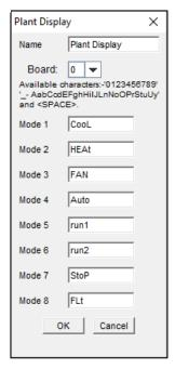
Within the fields 'Mode 1' to 'Mode 8', four alphanumeric characters can be inserted. The Available characters are listed within the properties box.
