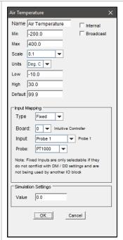
Fixed inputs are the device's or Expansion board's builtin Inputs.
