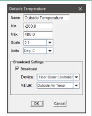
The properties box will allow details concerning the blocks name, min and max values along with units to be configured.
