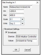
Now edit the TDB program in the TDB device you wish to receive the analogue value. Insert a Network Analogue Input block into the program and view the properties for this block as shown on the left.
