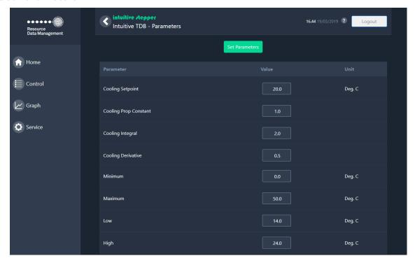
Clicking on Parameters shows a list of the current operating setting block values within the Data Builder (TDB) program. The user can change TDB program parameters from this page.
