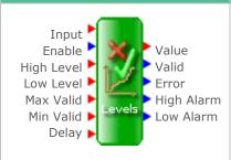
A Level block is used to monitor an analogue input and check that it is within pre-set parameters.
