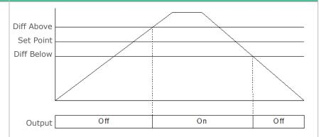
A Direct On/Off block works in the opposite manner to a Reverse On/Off block and would typically be used to control a cooling function.
