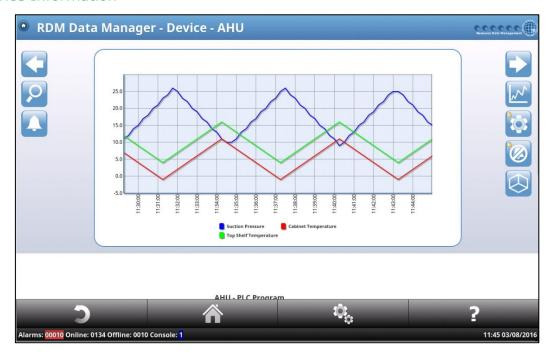
Pressing on the controller name will show the screen above. A dynamic graph displaying the last 15 mins will be at the top of the page and by scrolling down the user will see the inputs and outputs of the device (picture below).
