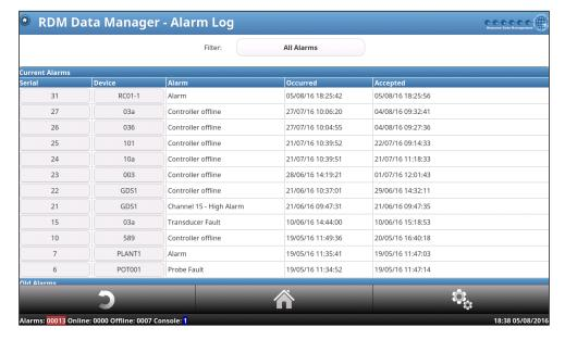
At the top of the screen any current alarms will be displayed with the old alarms underneath. There is a filter at the top that allows the user to view All Alarms, Current Alarms or Old Alarms.
