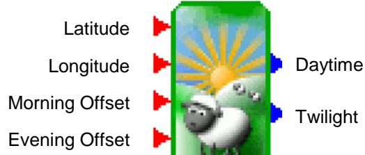
The TDB software application has a daylight block which can be used in conjunction with the light level sensor. By entering the latitude and longitude of any location the Daylight block can be used to provide an indication of daylight and twilight hours for a given geographical location.
