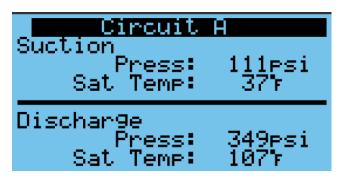
Active Protection Mode Screen. Shows the status of protection loops. If the system determines that there is a too high discharge temp, a too low suction temp, a too high suction temp, or a too low coil fin temp, the unit will automatically scale back the compressor or the fan in order to continue to operate without cutting off completely. If the main screen displays that a protection mode is active, this screen will identify it.
