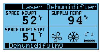
**Dehumidification Screen.** Shows information for assessing current status of the space and the dehumidification operation of the unit.
