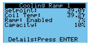
Compressor Request Screen. Shows if the compressor is on and what capacity it is currently commanded to operate at. The compressor will always be regarded as Ramp 1 and will be on Circuit A.
