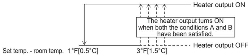
1st heater: Heater output from CN24-1(yellow) on the indoor unit control board.
